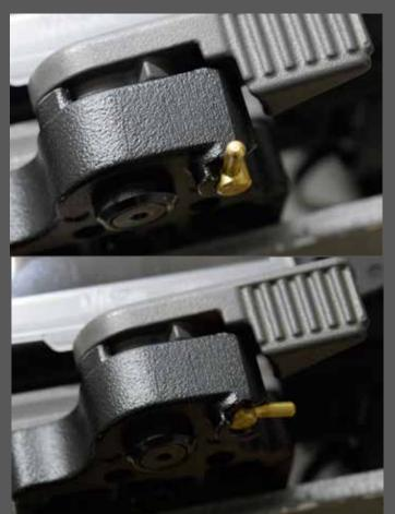
If you wish to remove the camera again, first turn the golden security lever upward. Now hold the camera tightly with one hand while pulling the grey locking lever upward. The camera disconnects from the adapter.
